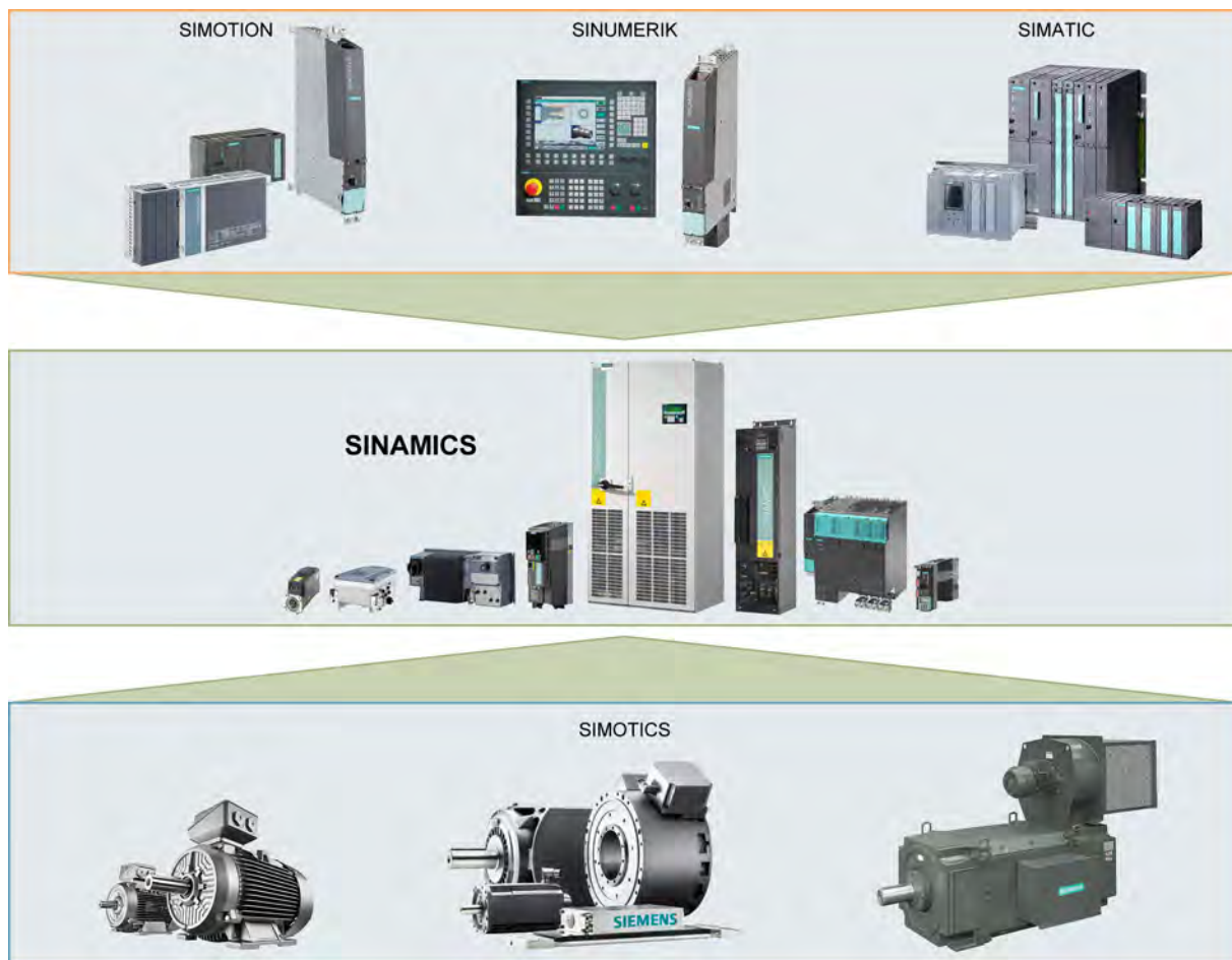
Figure 3-1 SINAMICS as part of the SIEMENS modular automation system
