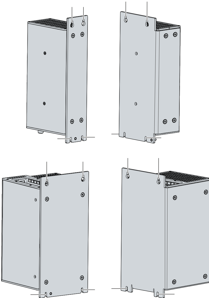
Fig. 21: C6920_Dismantling the control cabinet
