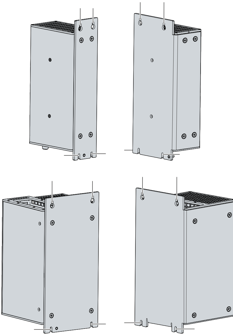
Fig. 16: C6920_Control cabinet installation
