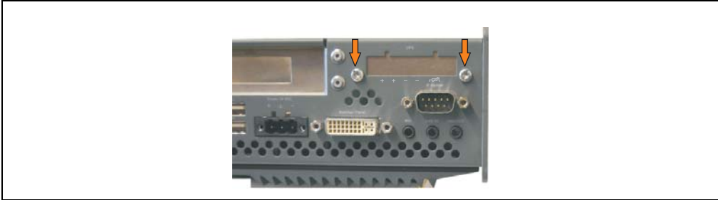
Figure 440: Remove UPS module cover
