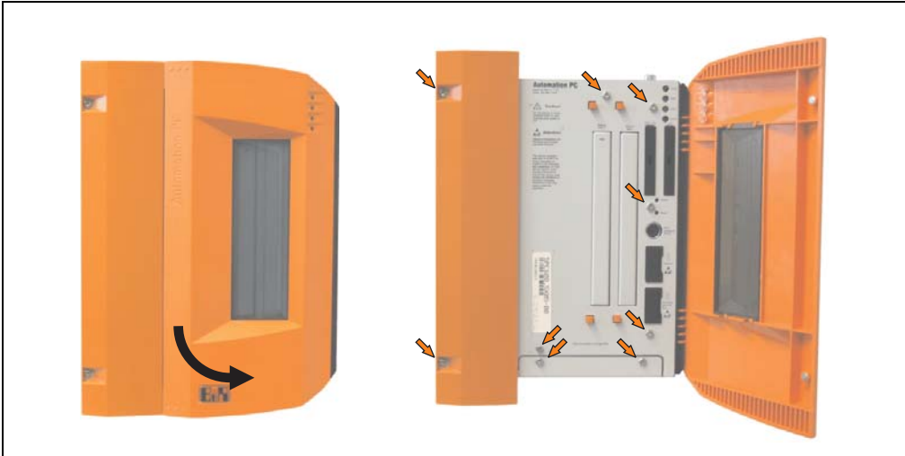
Figure 408: APC620 5PCI slot - Remove screws to install/ remove filter kit
