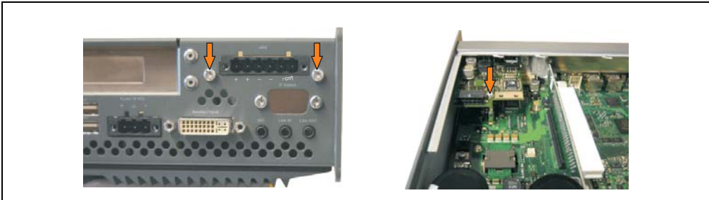
Figure 423: Install UPS module
