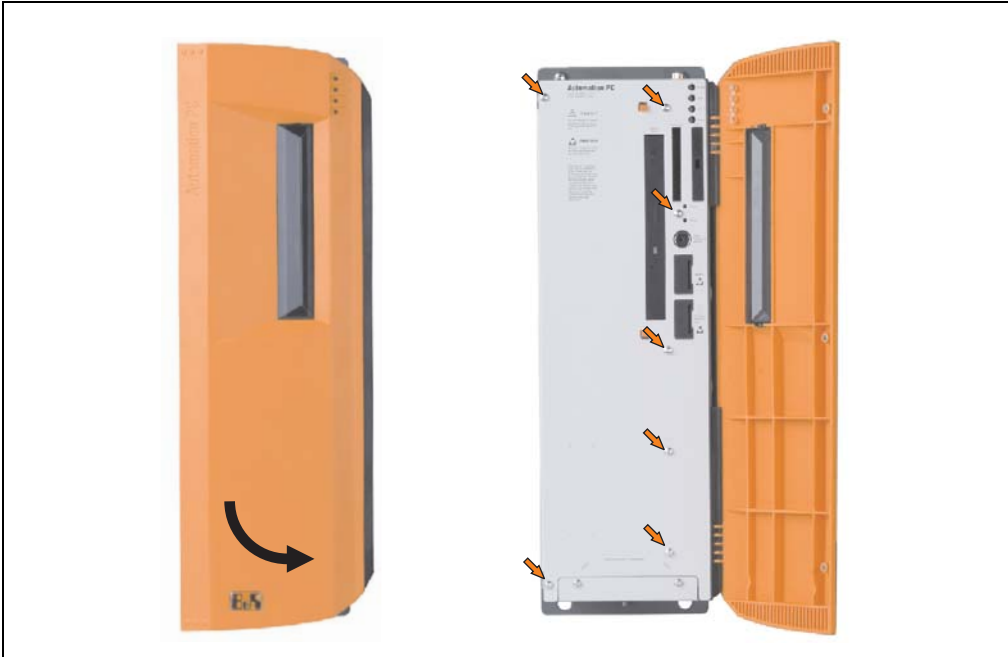
Figure 461: Mounting the side cover - APC620, 3 PCI slot
