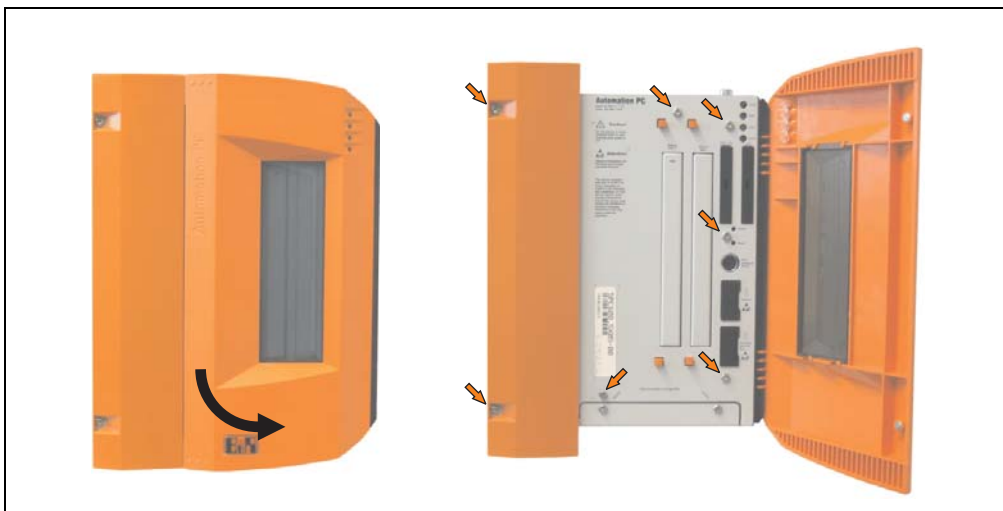
Figure 462: Mounting the side cover - APC620, 5 PCI slot
