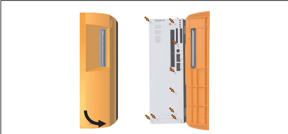
Figure 402: APC620 3PCI slot - Remove screws to install/ remove filter kit
