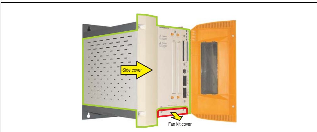
Figure 409: APC620 5PCI slot - Remove side cover and fan kit cover
