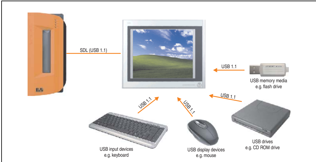
Figure 169: Remote connection of USB peripheral devices to the APC800/900 via SDL
