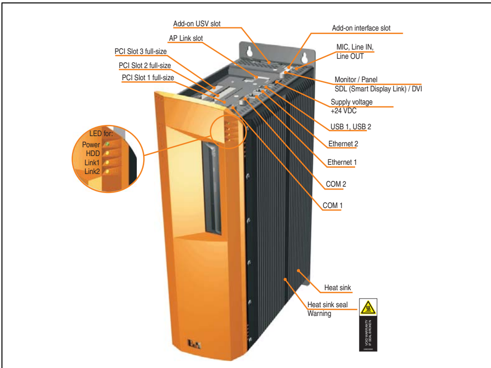
Figure 13: Interface overview - APC620, 3 PCI slot variant (top)
