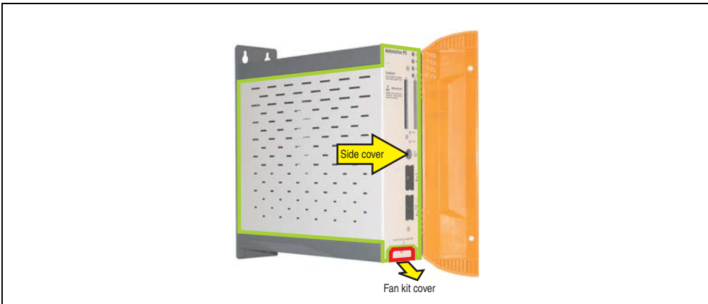
Figure 392: APC620 1PCI slot - Remove side cover and fan kit cover
