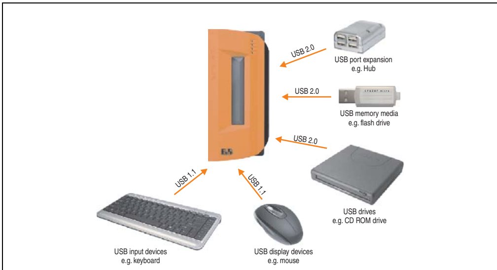
Figure 167: Local connection of USB peripheral devices on the APC620
