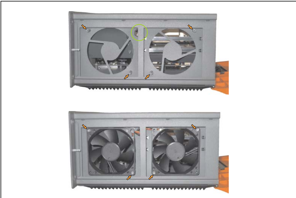
Figure 405: APC620 3PCI slot - Fan installation
