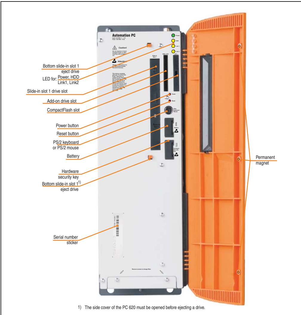
Figure 14: Interface overview - APC620, 3 PCI slot variant (front)
