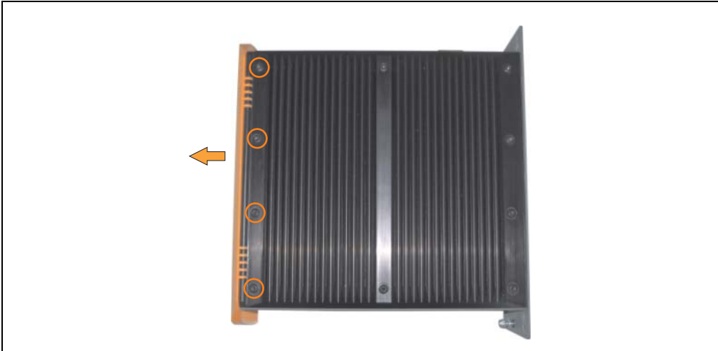
Figure 465: Removing the APC620 front cover
