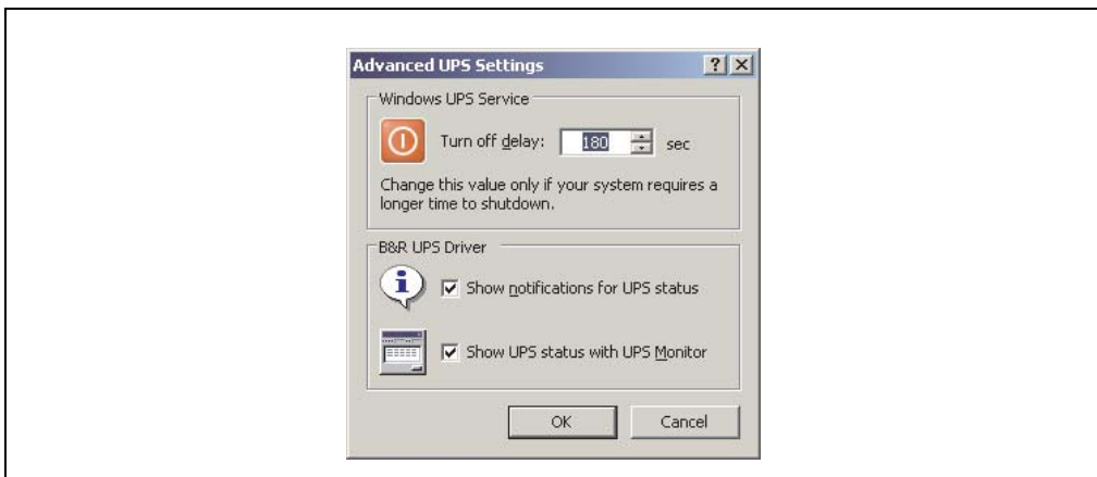
Figure 300: ADI Control Center - Advanced UPS settings
