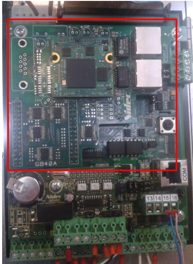
Figure 2.7.5: GB40A-PROFINET - GB40A-EtherNet/IP optional board mounted on BASIS control board
