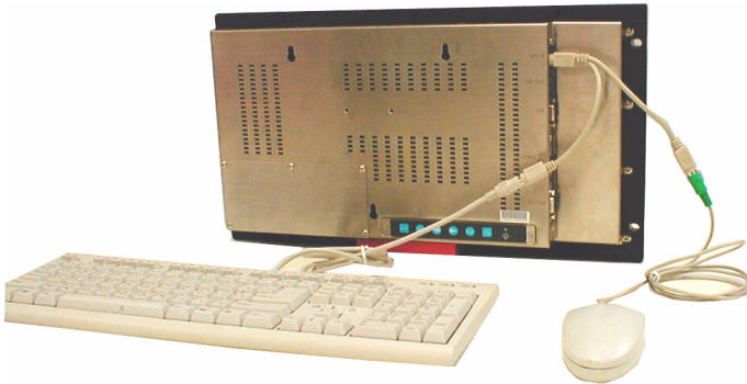
Figure 2.4: Connecting Back External Keyboard/Mouse
