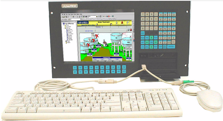
Figure 2.3: Connecting Front External Keyboard/Mouse
