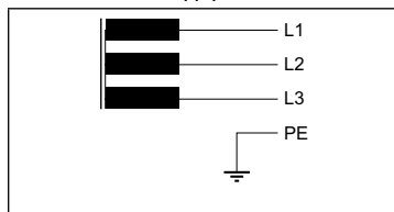
IT supply lines
