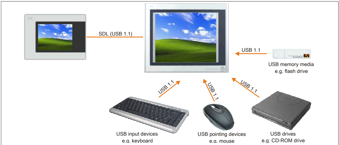
Figure 74: Remote connection of USB peripheral devices on the APC800/900 via SDL
