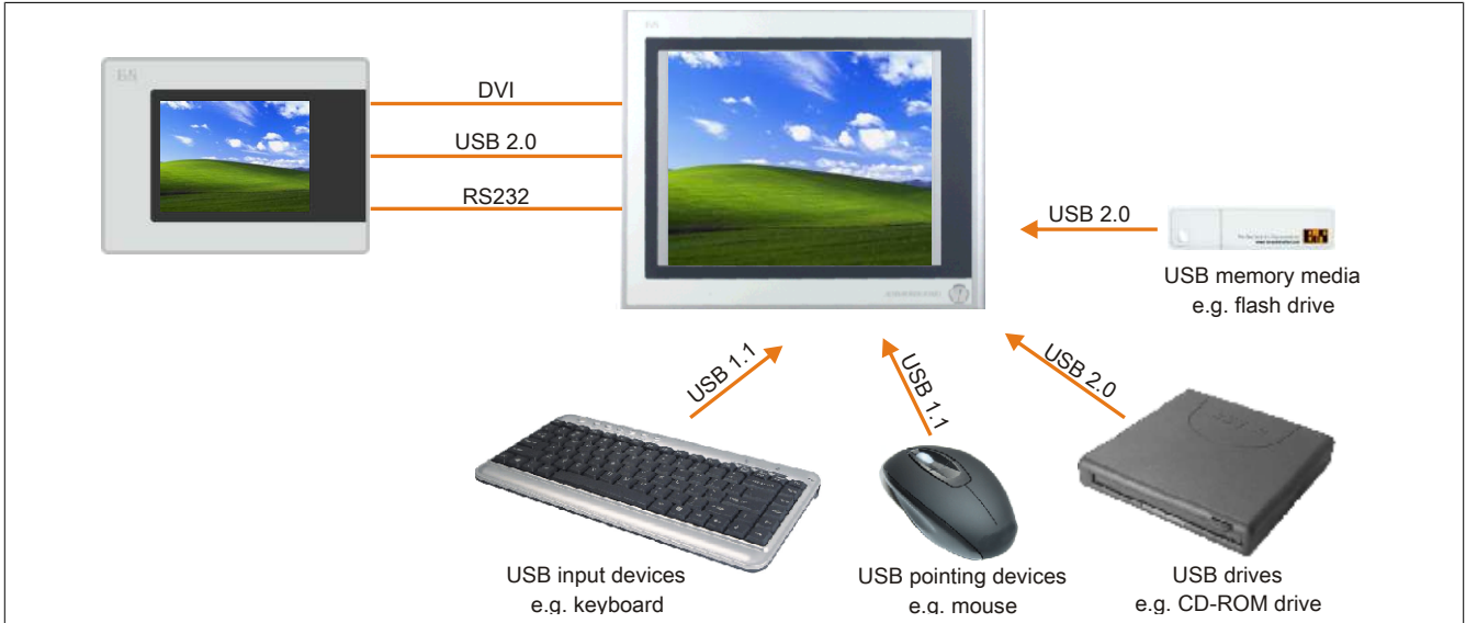
Figure 73: Remote connection of USB peripheral devices on the APC900 via DVI
