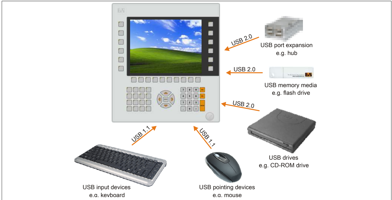
Figure 72: Local connection of USB peripheral devices on the PP500
